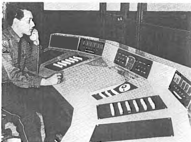
The Master Control Board enables one officer to operate all radio and telephone networks simultaneously at the new Communications Center
