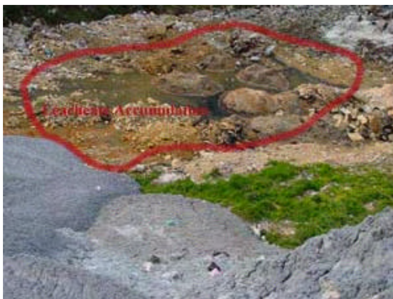
Photograph 6.1. Accumulation of leachate in the landfill during winter.
