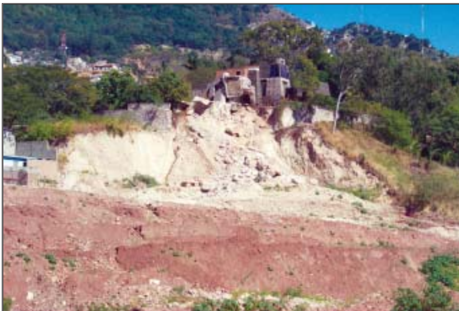
Figure 8. Debris slide at Barrio Mira Mesi that has progressed headward even during dry seasons following Hurricane Mitch despite the placement of a soil berm (shown in the foreground) to protect the slope.
