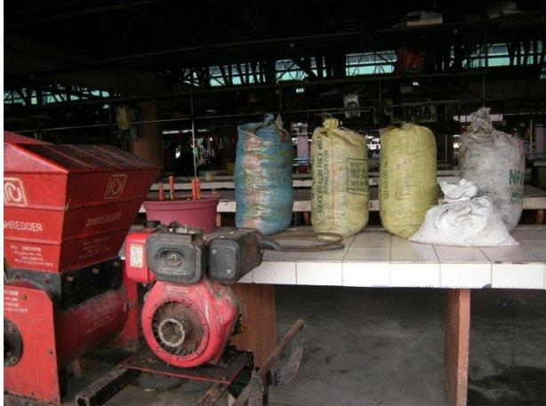
Shredder used to prepare compost
