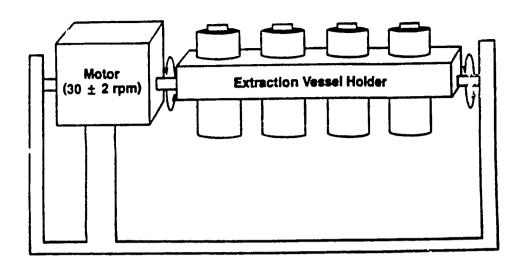
Figure 1. Rotary Agitation Apparatus
