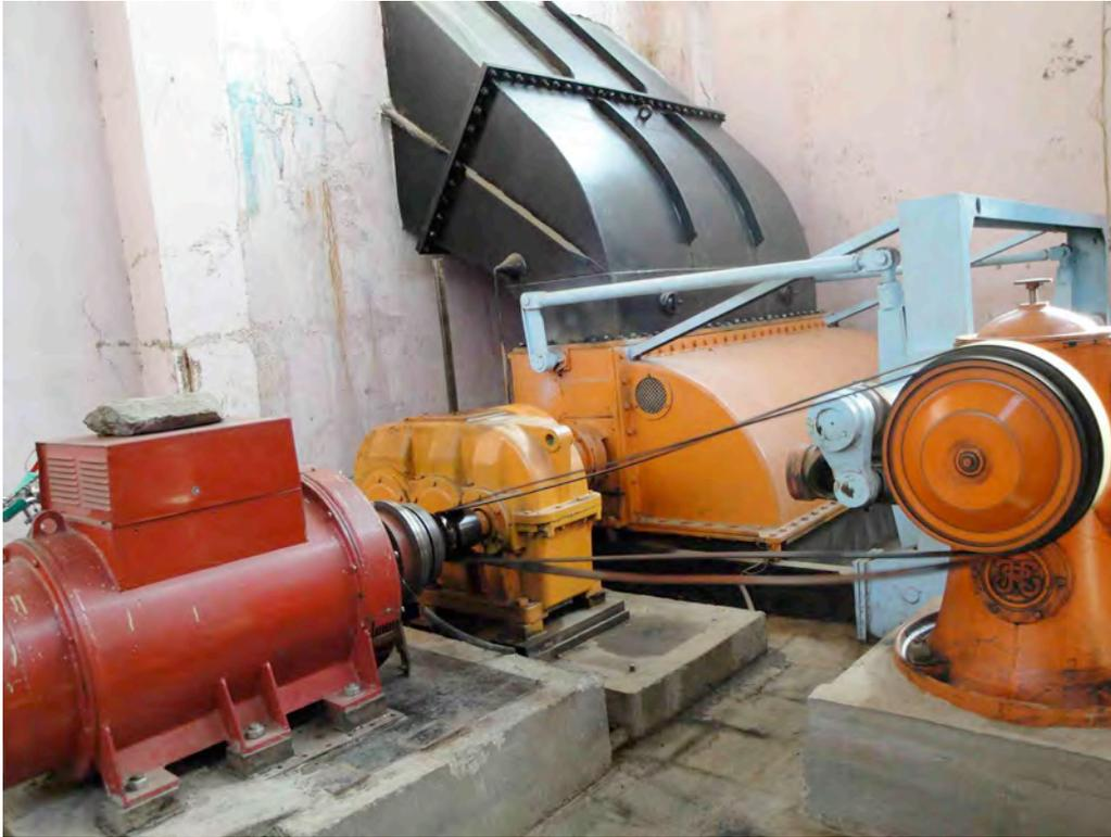
**Fig. 5. Asad-Abad turbine and generator (notice rock on top). The system should be rehabilitated to double production back to the original 700 kW power rating.**
