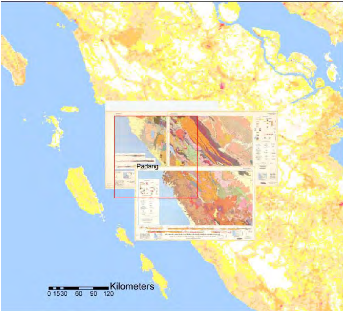
Figure 9. Map showing the three 1:250,000-scale geologic maps that were used as the basis for the shear-wave velocity ( V_{s30} ) characterization of the Padang region (red box). Maps are shown after scanning and rectifying these maps in GIS (see text).
