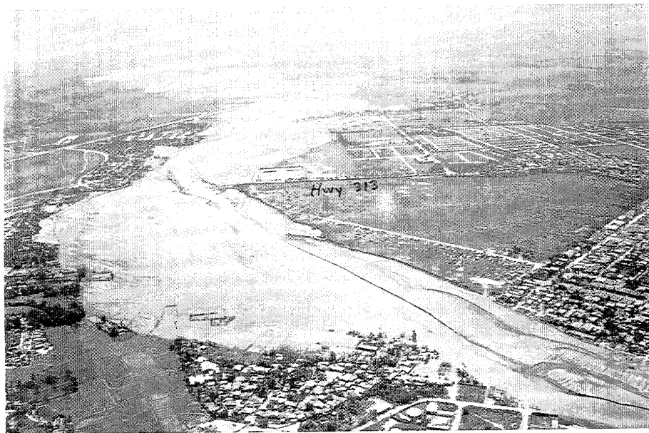
Bank erosion and sediment deposits downstream from Angeles City, September 1991.
