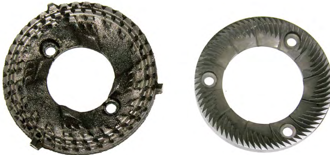
Figure 1: The Grindmaster grind burrs (left) break the coffee using teeth in a concentric circle, while most other grinders use blades that emanate radially from the center (right). Each type has its advantages, but they produce significantly different particle size distribution.
