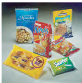
Multilayers from PE and PP
