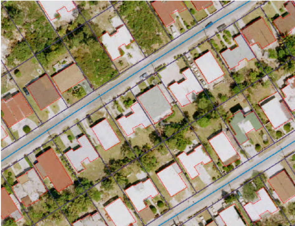
FIGURE 2. PINWOOD GARDENS SUB-DIVISION, NEW PROVIDENCE: EXAMPLE OF INTEGRATED SPATIAL DATA FOR LAND MANAGEMENT
