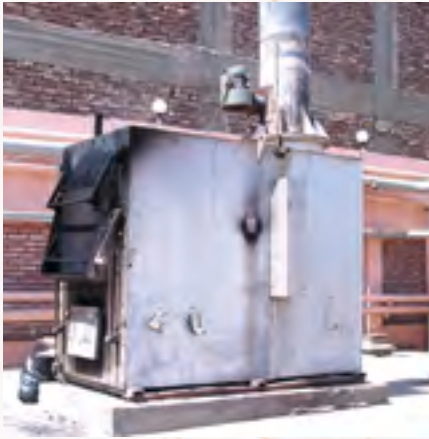
Incinerator for medical waste in Luxor.
