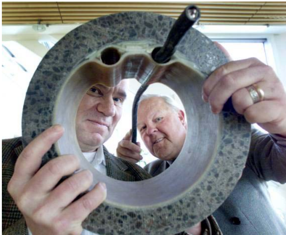
Figure 4.11: Fiber Cable as Part of Relining Leaking Sewers
