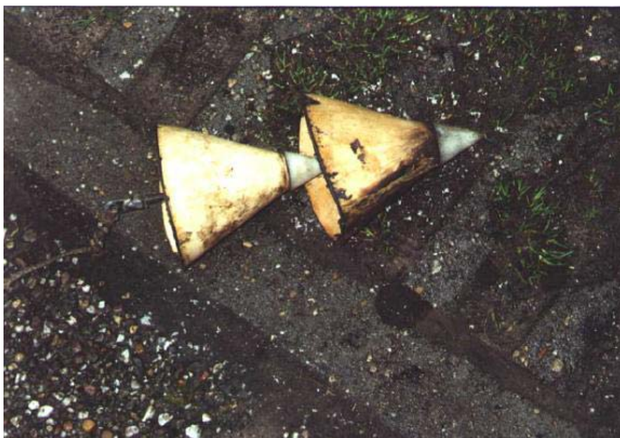
Figure 4.16: Shuttle Used by Gastec for Pulling Optical Fiber Conduit
