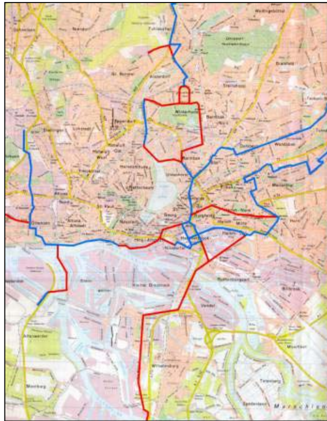
Figure 4.5: Fiber Network in Hamburg Sewers
