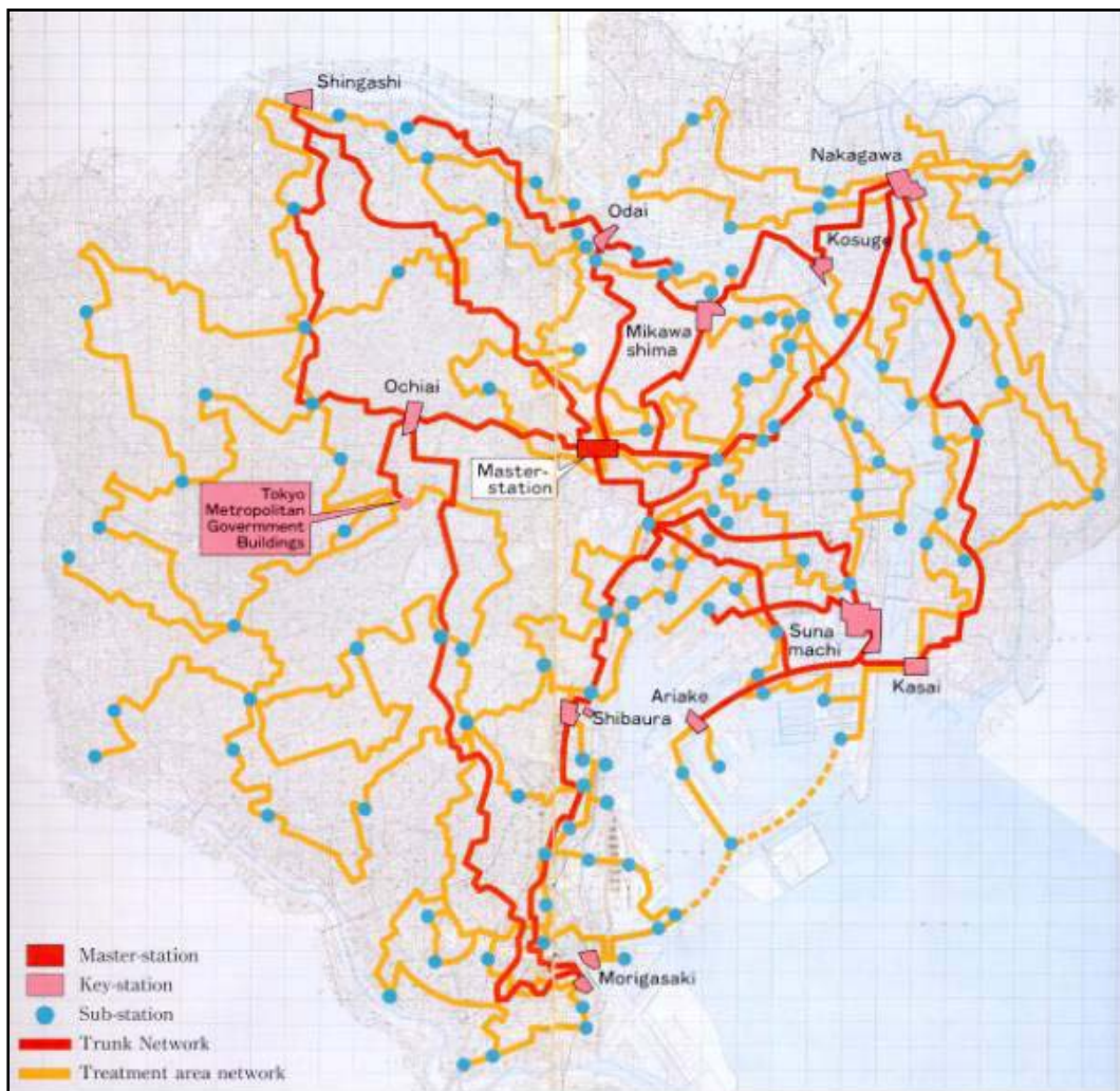
Figure 4.2: Optical Fiber Cable Network in Tokyo Sewers of Over 850 km
