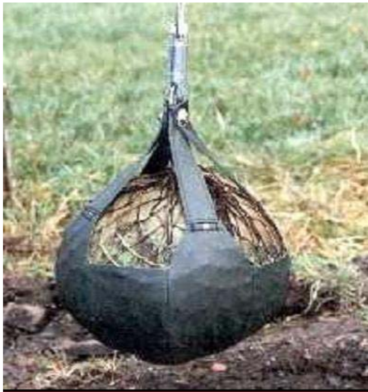
Figure 4.12: Special Balloon Used in Alcatel Gas Pipe Technology
