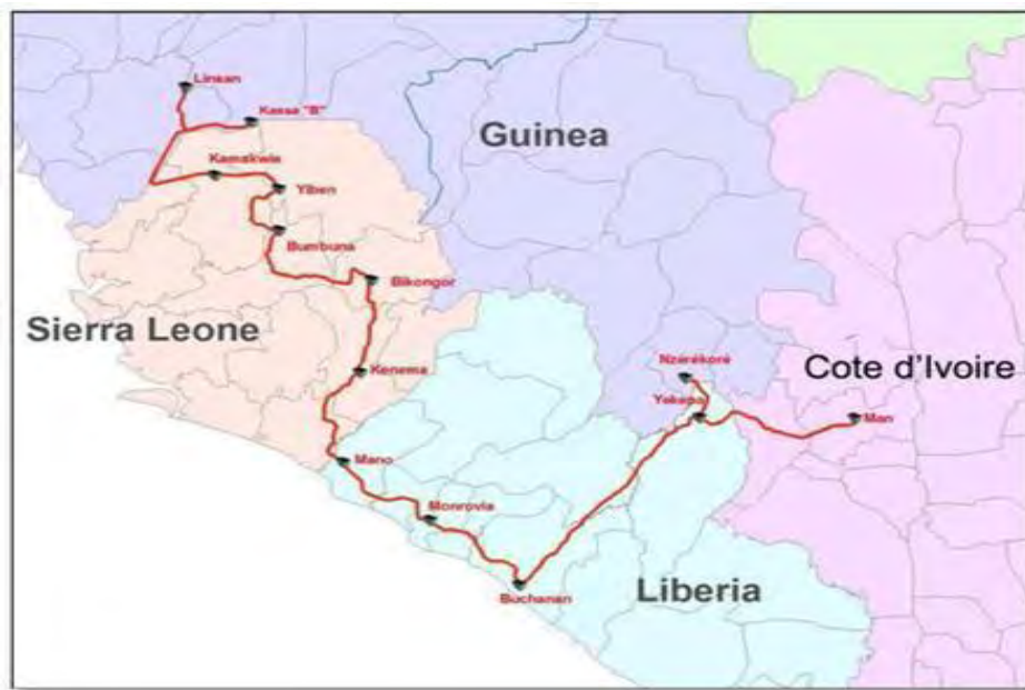
FIGURE III. CLSG 220 KV TRANSMISSION LINE ROUTES
