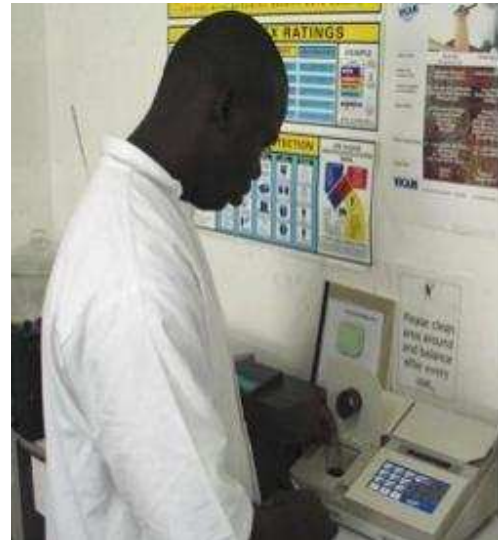
An FDD lab technician tests local peanut for Aflatoxins using equipment procured with GTIS funds. The FDD is now able to certify peanuts and peanut products for local consumption and export, benefiting both consumers and manufacturers.
