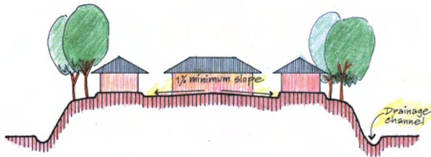
Fig. 6.2 Homestead design aspects and photo showing house in flood-prone area of Manikganj with screened off machan which is normally used for storage
