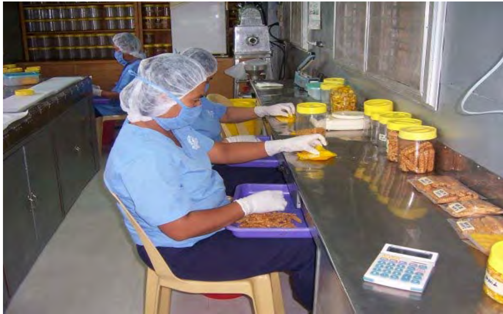
Fig. 13 Packing of peanut brittle in cellophane as its primary packaging and in polypropylene jars as its secondary packaging.
