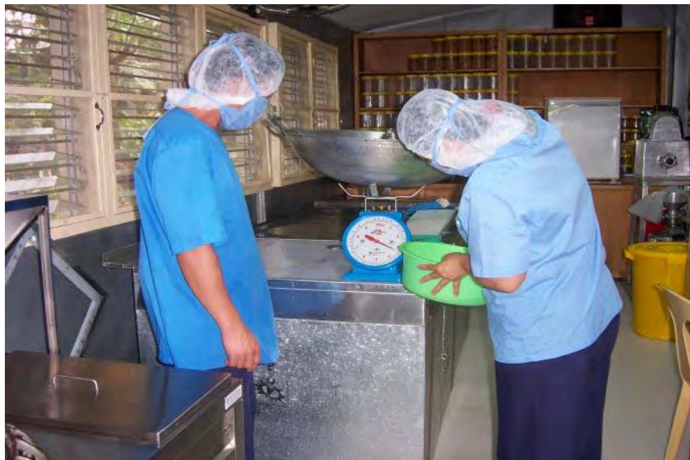
Fig. 8 Weighing of glucose syrup directly on the cooking pan due to its thick consistency.
