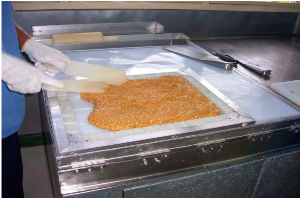
Fig. 10 Molding and flattening of hot peanut brittle mixture in a pre-formed molder made of plastic formica with grids.
