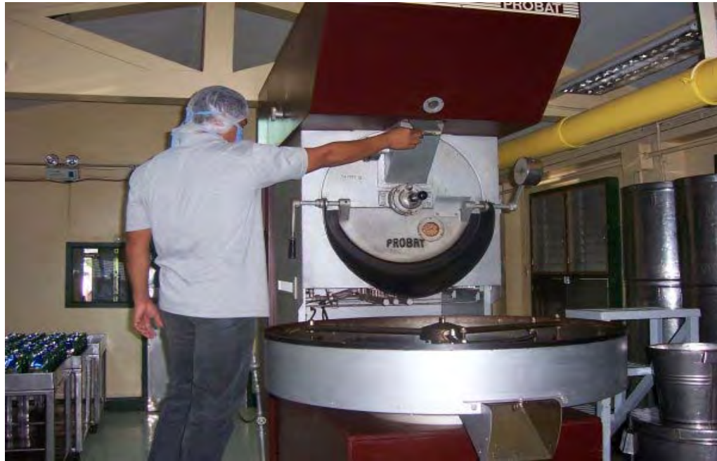
Fig. 1 Dry blanching and roasting of peanuts are performed in a Probat coffee roaster at 149°C.
