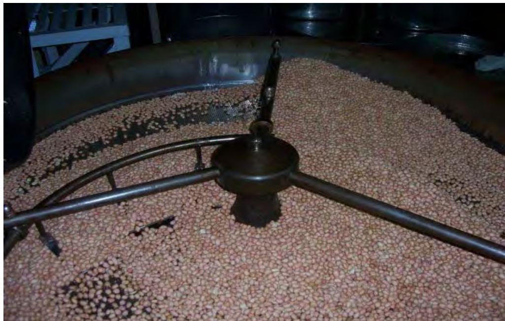
Fig. 2 Cooling of peanuts using the paddle of the roaster and air from the roaster that sucks out heat from peanuts.
