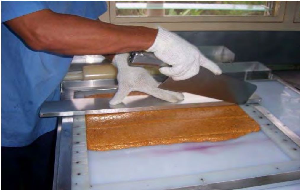
Fig. 11 Cutting of peanut brittle mixture.
