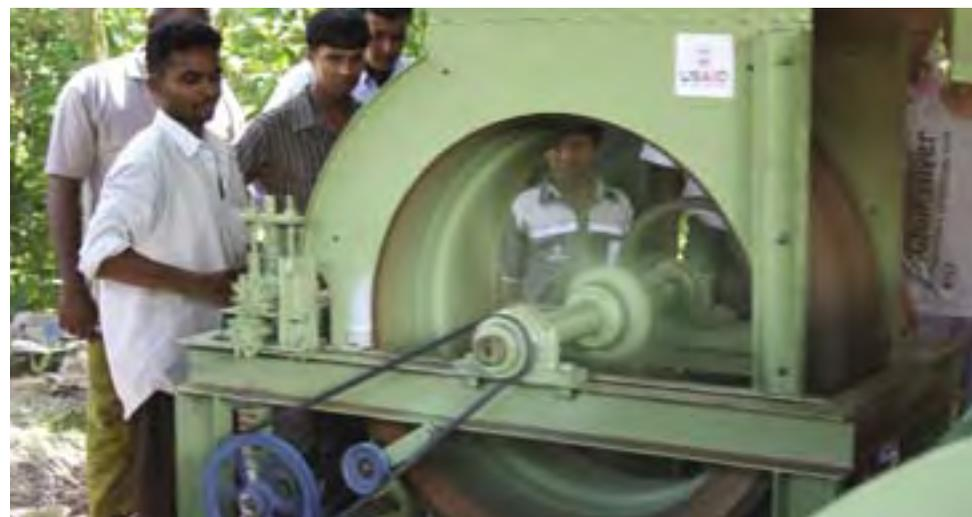
A local tradesman demonstrates the new decorticator, which vastly reduces the time it takes to remove husks from coconut shells.
