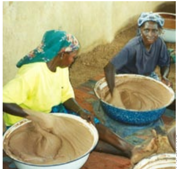
Processing shea butter requires kneading by hand to separate the fat from the other parts of the kernel.
