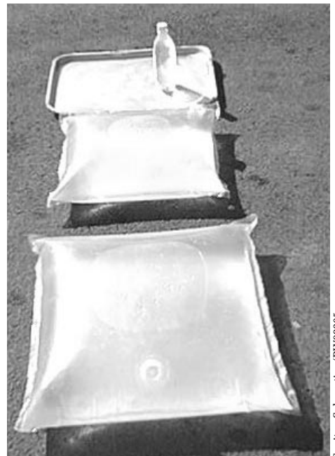
Figure 2.3. Solar water disinfection in the Caribbean.
