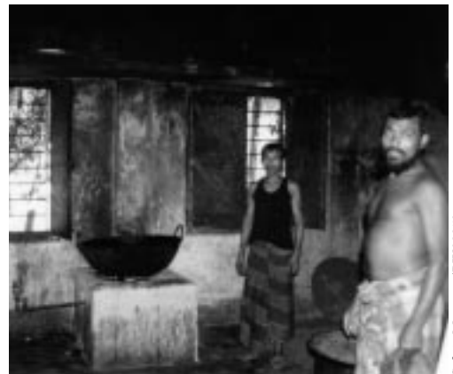
Figure 6.10. Oven fueled by biogas.
