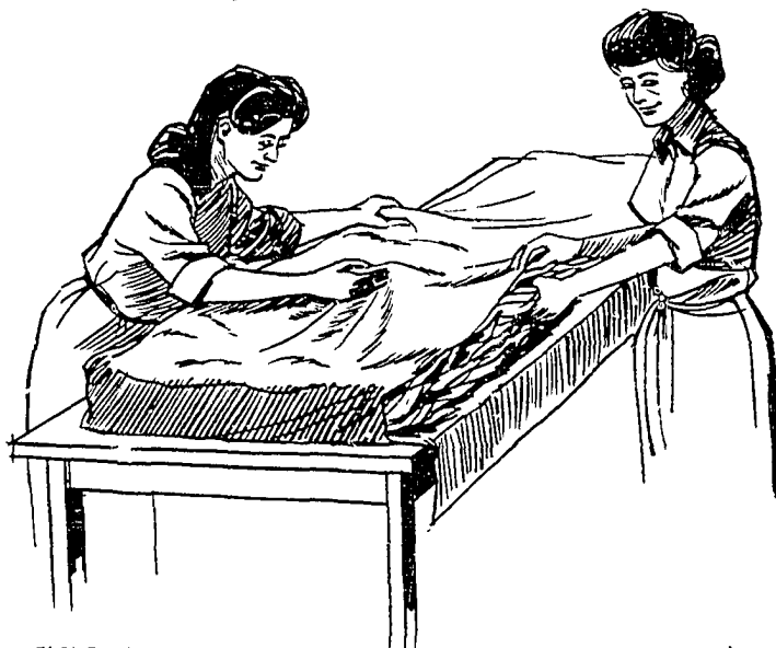
FIGURE 3. CORN SHUCKS OR SIMILAR FILLING MATERIALS ARE STUFFED INTO THE COVER, WHICH IS MADE FROM SIX PIECES OF CLOTH SEWN TO FORM A BOX WITH SQUARE CORNERS.
