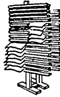
FIGURE 5. A SIMPLE DRYING RACK CAN BE MADE FROM 5 CM X 5 CM UPRIGHTS WITH 2.5 CM X 2.5 CM CROSSBARS ABOUT 2.5 CM APART.
