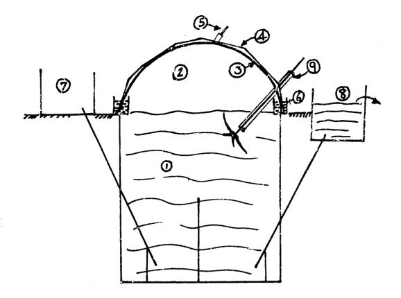
time and a significant reduction in the size of the digester. This "ASTRA" model reflects IIS studies on the optimization of digester dimensions which indicated that the diameter of the digester should be at least equal to the depth of the slurry chamber. The diameter of the pilot unit was 1.83 m, while the depth of the chamber was only 1.62 m. The ASTRA model has not yet been widely used in India.
