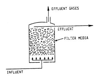
A great variety of non-biodegradable materials have been used as packing media for anaerobic filter reactors including various types of stone, several clay and ceramic materials, plastic shapes, coral, mussel shells, reeds, and bamboo rings. The most desirable characteristics of the media are a large surface area and a porous surface to which the microbes are easily attached.
