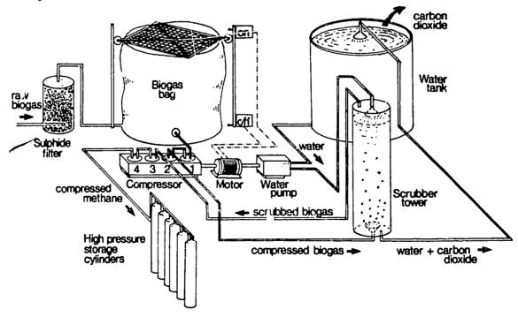
the CO<sub>2</sub> in the biogas dissolves easily in water under pressure, as in carbonated soft drinks, while the methane rises to the top of the tower. The water with dissolved CO<sub>2</sub> flows to an open tank where it loses pressure and the CO<sub>2</sub> is released to the atmosphere. The scrubbed biogas is now 95% pure methane. (See March 1983 Bioenergy Systems Report, pp. 16-17, on removal of hydrogen sulphide from biogas prior to use in engines.)
