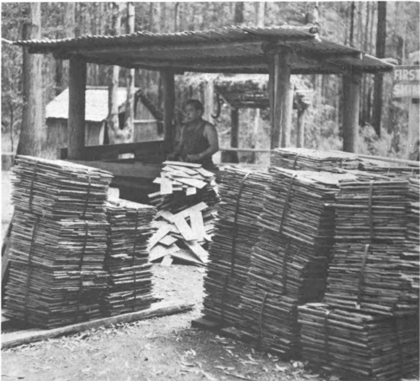
Roofing. Roof shingles being cut from Casuarina torulosa near Wauchope, New South Wales, Australia. (CSIRO Division of Forest Research)
