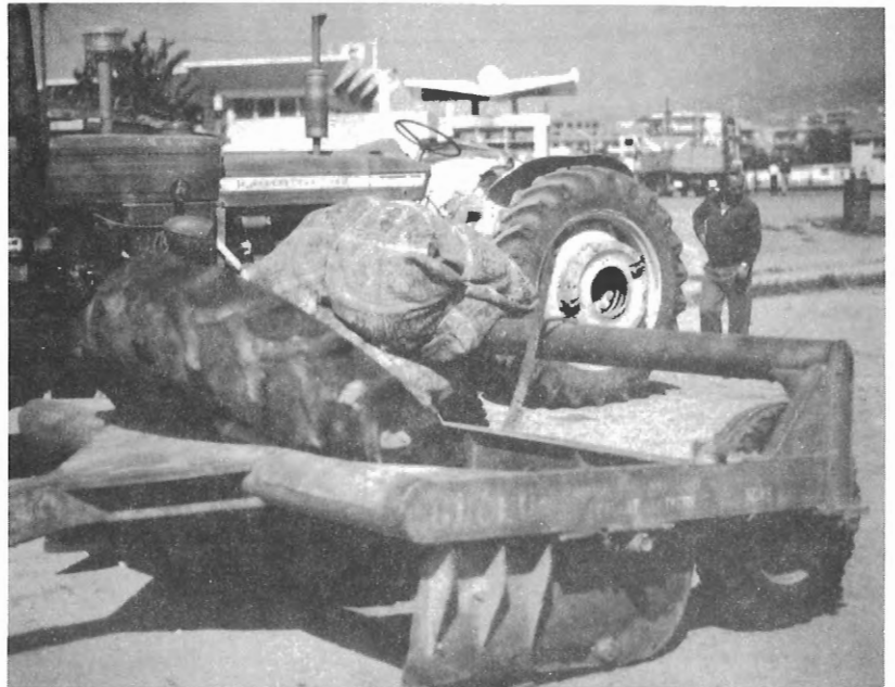
Old mechanical scraper manufactured during the project which is still used by private contractors.
