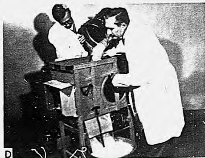
Figure 3.--Processing whole soybeans: A, cooking; B, air-drying; C, cracking cooked, dried beans; D, winnowing to separate hulls; E, diagram of winnower construction and operation; and E, hand grinding meats to flour.
