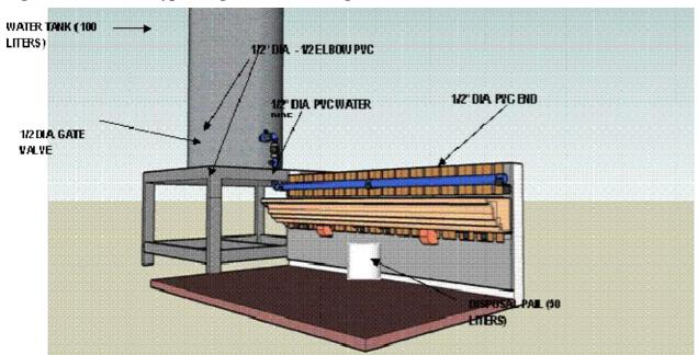
Figure 2. Classroom-Type Design of Handwashing Station
