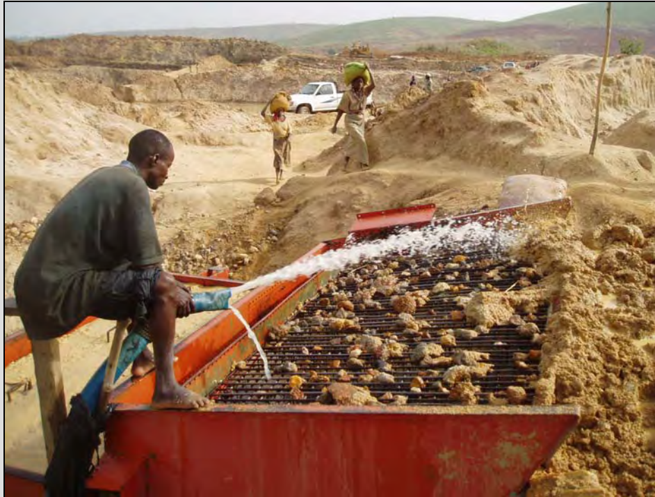
Gravel washer and two gravel carriers at a semi-industrialized diamond mine in Banankoro
