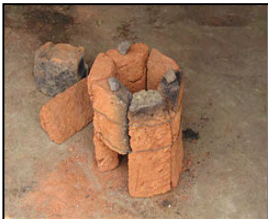
Photo 5.8: Basic construction of a six-brick stove before it is plastered with clay
