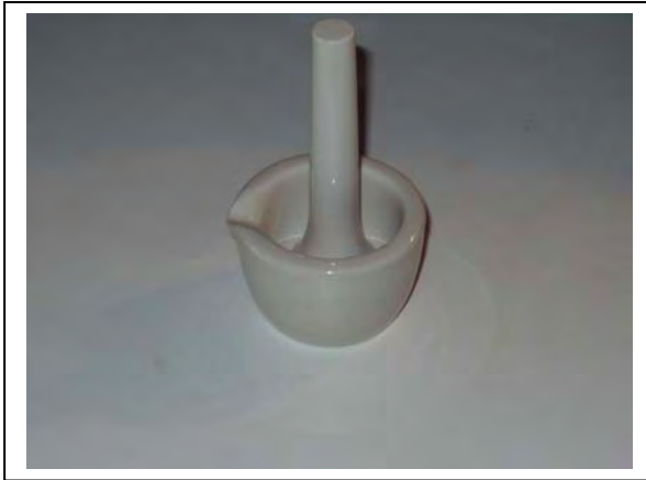
Figure 12. Pour liquid nitrogen into the mortar/pestle configuration and fill to the brim of the mortar
