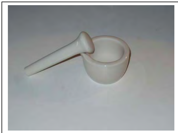
Figure 13. For the third filling of liquid nitrogen into the mortar, remove the pestle and rest the pestle on the lip of the mortar.
