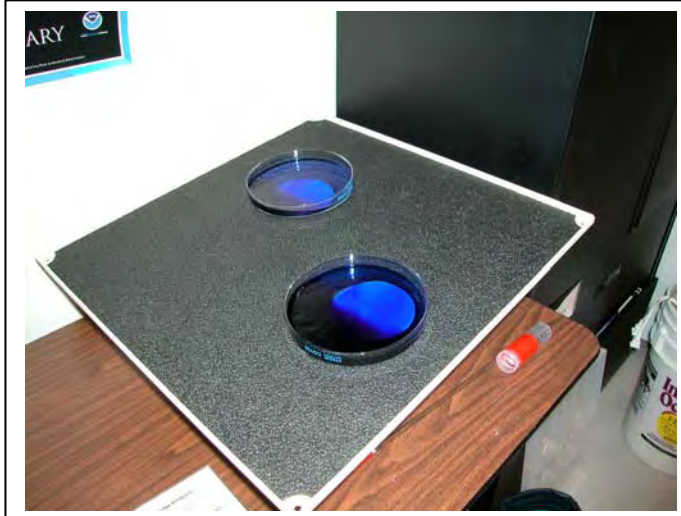
Figure 20. Incubate the filter paper in an incubation boat. The boat can be anything: e.g., petri dish or weigh boat, and be made from plastic or glass. Stain solution should cover the filter paper either in its entirety or so that each rocking slant covers at least 50% of the filter paper in the Stain Solution.
