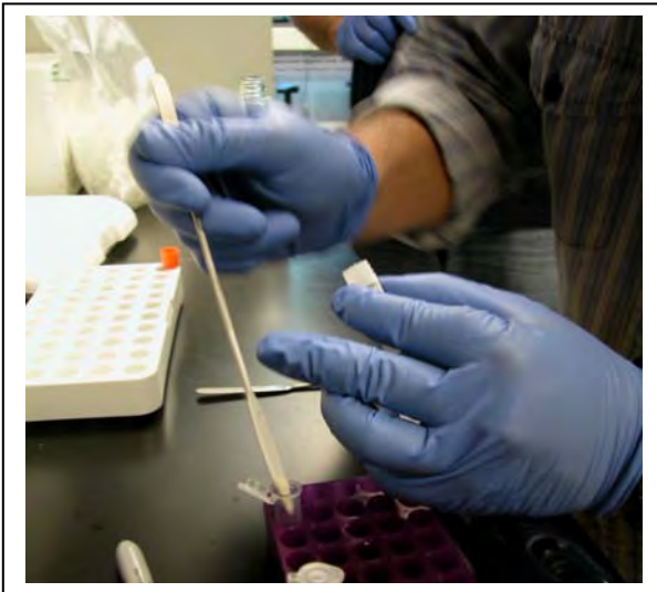
Figure 16. Remove frozen, pulverized sample from cryo-vial with a pre-chilled spatula. Place sample on spatula into a locking microcentrifuge tube. Photograph courtesy of Phillip Dustan.
