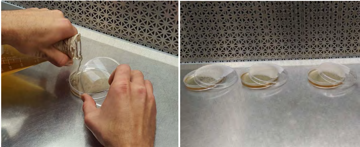
Photo 2: Left) Hot agar is poured into petri plates in a layer about 0.5-0.75 cm thick. Right) Hot agar petri plates are propped open and left to cool in the laminar flow cabinet to prevent condensation buildup.
