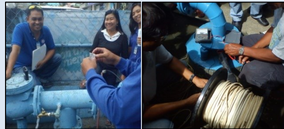
Demonstration on monitoring and testing of chlorine residual of water
