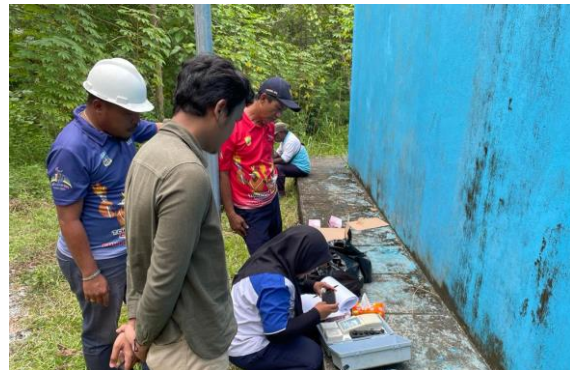
As part of the WSP training, the training participants in Jayapura practice testing the quality water at Sentani water supply system intake.
