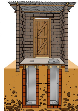
Figure 5. Alternating lined pits with a pole interface or a pre-cast concrete slab interface for high water table and areas with loose soil formation
