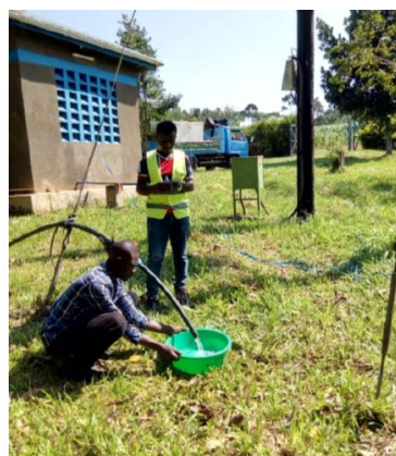
Figure 2. Yield measurement. The abstracted water was disposed away from the borehole to avoid recirculation.
