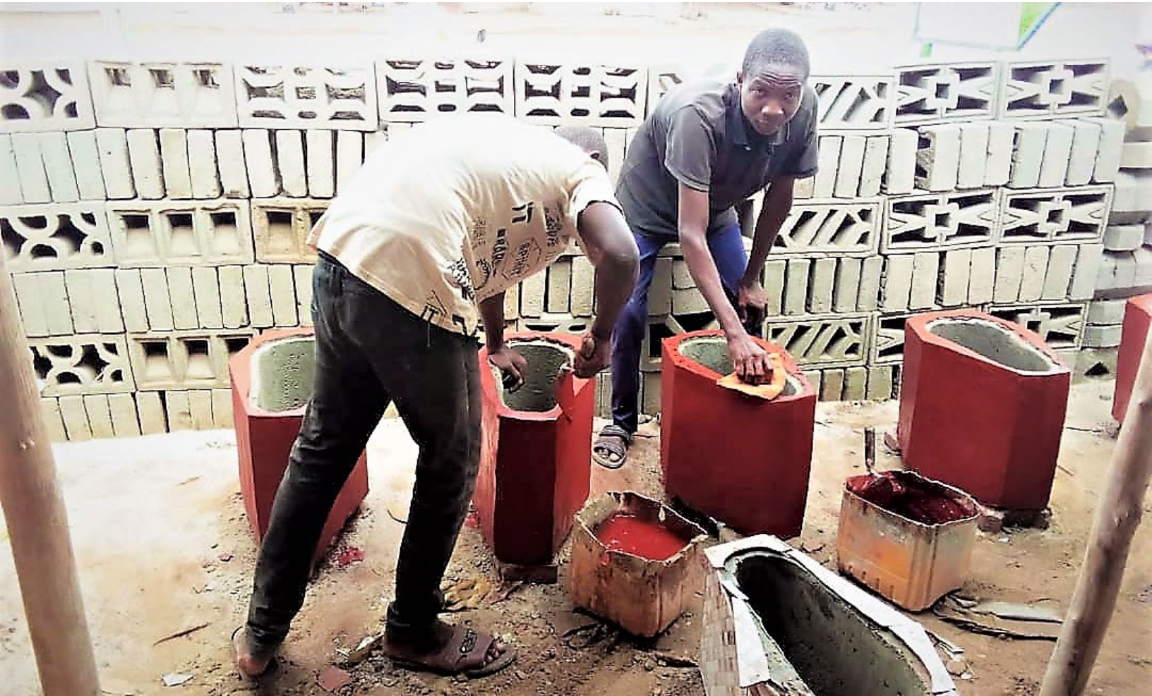
A mason building seated toilets © MuniWASH Benin
