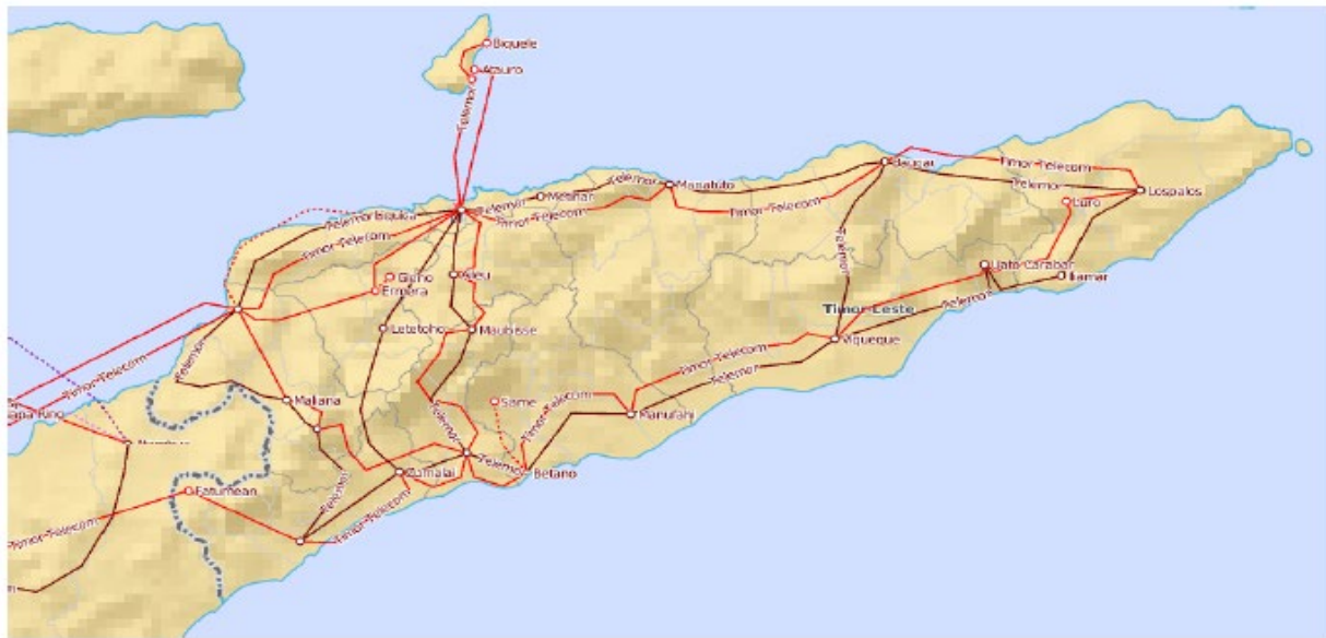
Figure 4: Timor-Leste's fiber-optic infrastructure. The solid red line depicts operational microwave, the dashed red line depicts planned microwave, and the brown line depicts operational fiber-optic cable. (ITU and ESCAP, 2019)
