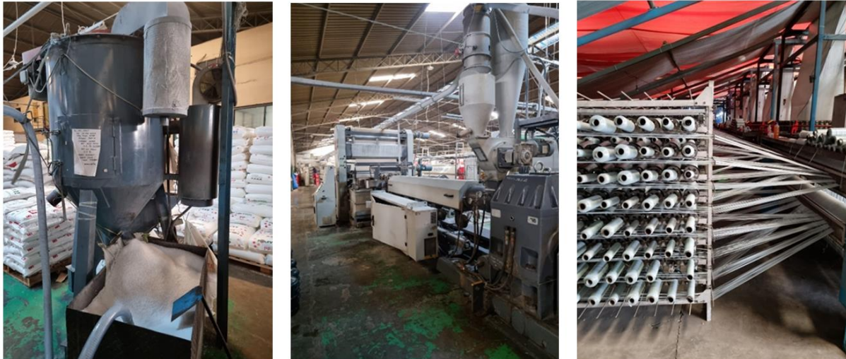
The hopper (left), extrusion machine (middle), and tapes (right)
