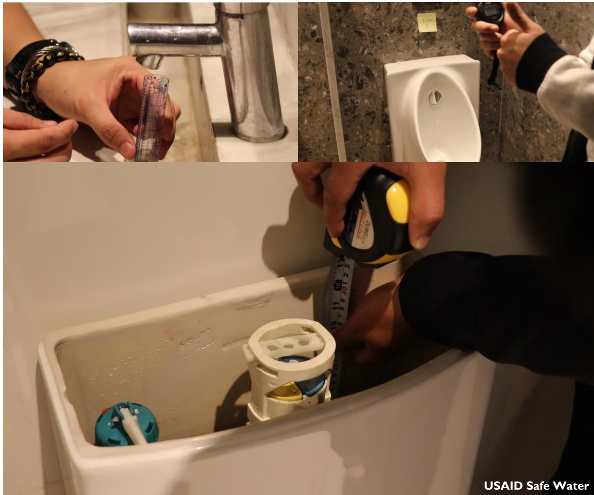
Actual Water Audit. (Counterclockwise; 1) A drip vial is used to measure the leakage in a faucet. Participants calculated the liters of water that’s wasted by the leaking faucet using a formula taught during the training. (2) A participant shows a thumbs-up sign as he clicks the stopwatch after the urinal flush is completed. Another participant records the time and compares this with the industry-acceptable standard to check for water efficiency. (3) A participant measures the depth of the water closet of a dual-flush toilet as part of calculating the water efficiency of the toilet bowl.
