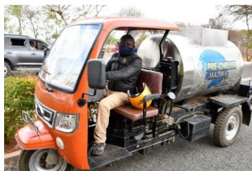
An 800-liters mobile solar-powered chiller from Savannah Circuit Technologies Ltd. Photo credit: KCDMS
