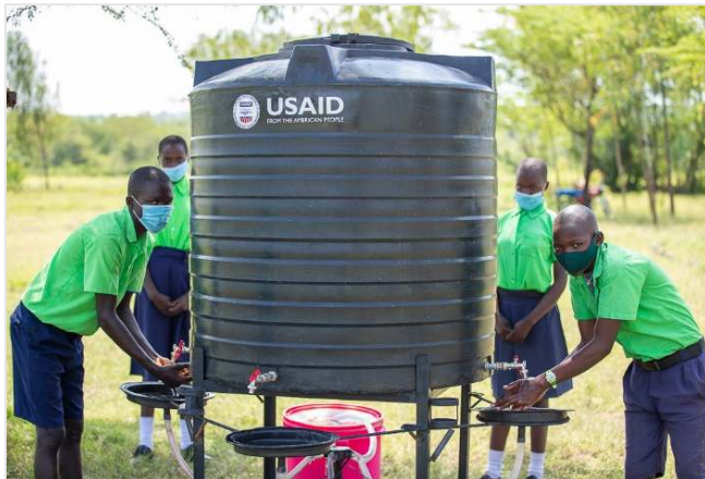
Pupils using a handwashing station supplied by KIWASH. Each school received a multi-user handwashing station while health facilities/border points received single-user foot-operated stations.
