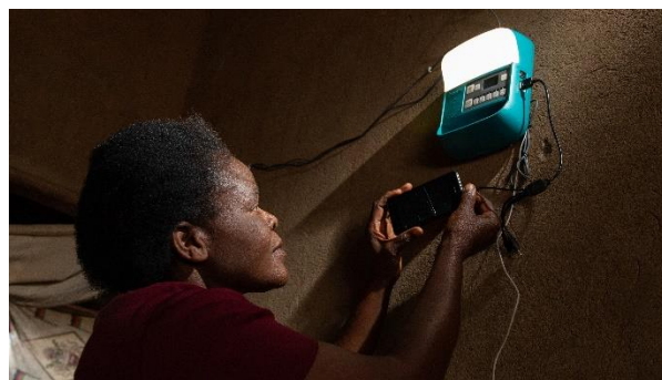
Most SHSs have small radio and mobile phone charging devices that are powered by a solar panel and battery. Photo credit: USAID SAEP
