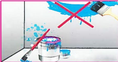
Avoid painting, washing or covering the sprayed walls for at least 8 months after spraying
