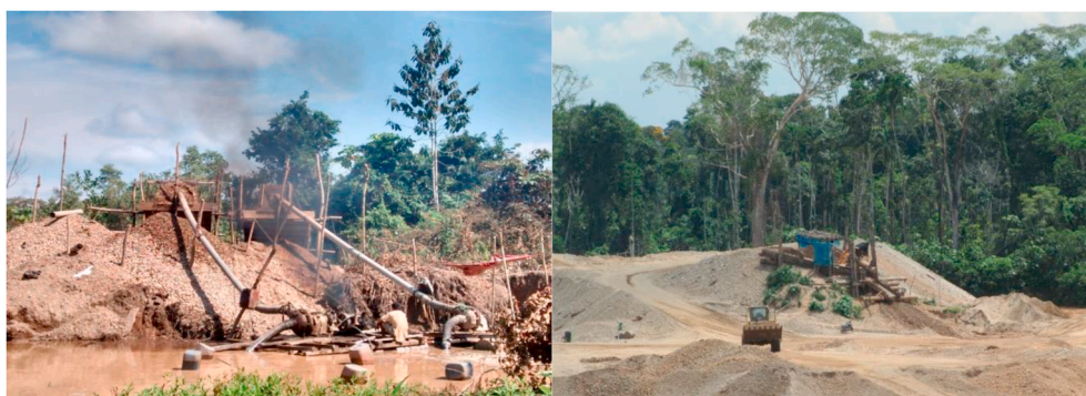
Fig. 2. Technologies to extract sediments: minimally mechanized mining (left) and highly mechanized mining (right), located in Laberinto district and Kotzimba Native Community in the Peruvian Amazon, respectively.
