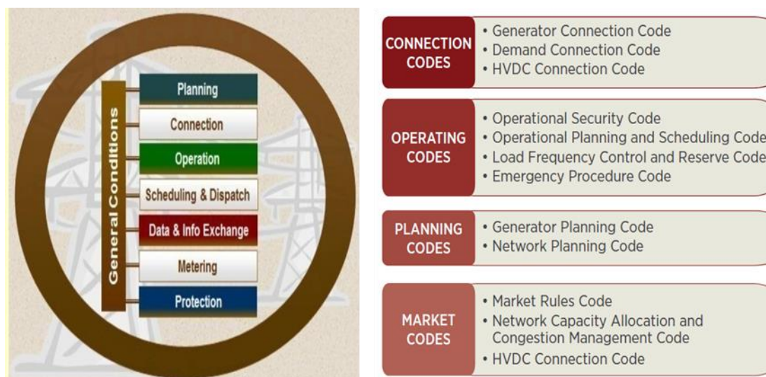
Figure 1. Grid Code Structure and Types of Codes that Form a Grid Code
