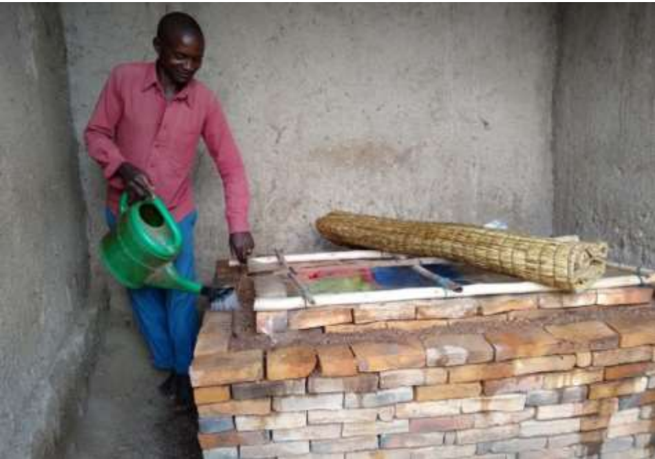
Figure 2. Manual watering of the sand and brick of a ZECC to activate evaporative cooling for fresh produce storage in Rubona, Rwanda. (Source: Feed the Future Innovation Lab for Horticulture, 2019)
