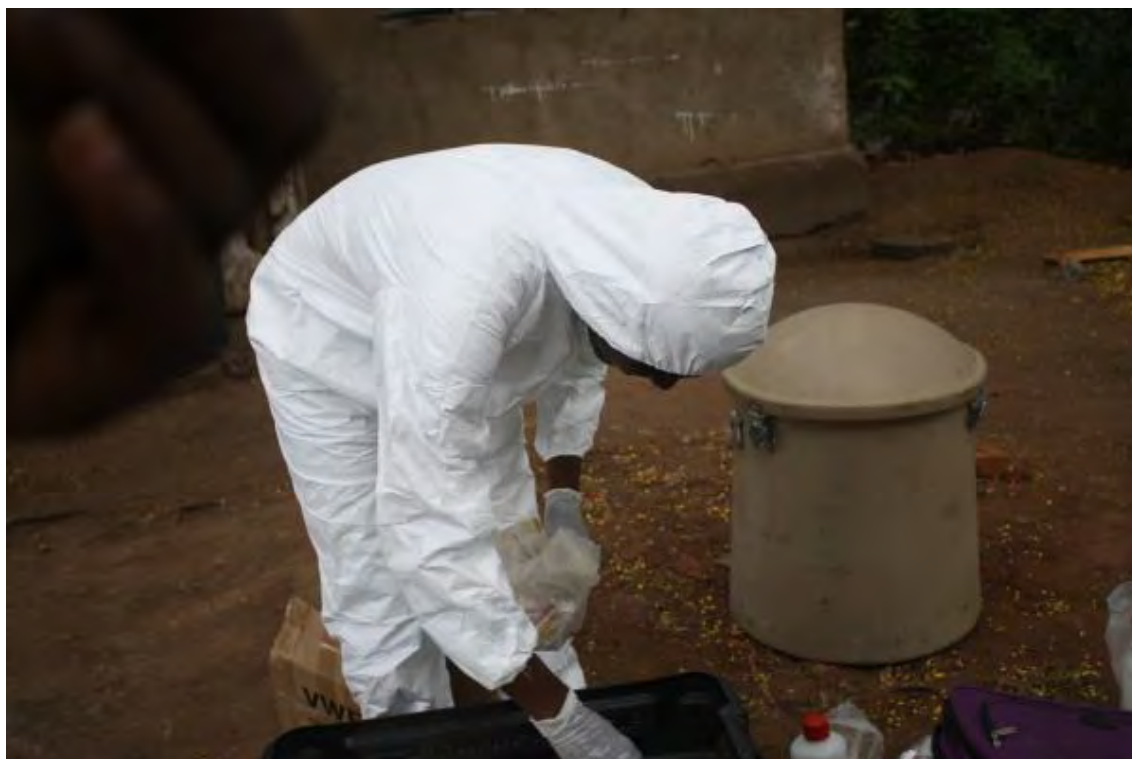
Figure 1: The PREDICT Tanzania team packs up equipment after collecting specimens from rodents. The mushroom shaped container in the background is a specially designed transport container for LN2 dryshippers, ensuring the dryshipper container is well protected during overland or air travel, and that all stored specimens are well within the temperature range required for viral isolation. Photo by Liz Vanwormer.
