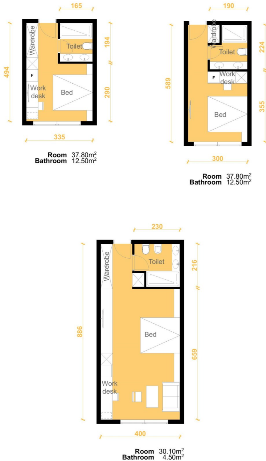
Figure 31 –Sample of the guestroom layout based on the minimum requirement set in Gazette (No.1963/28 of 20th April 2016) and Board Approved Guidelines
