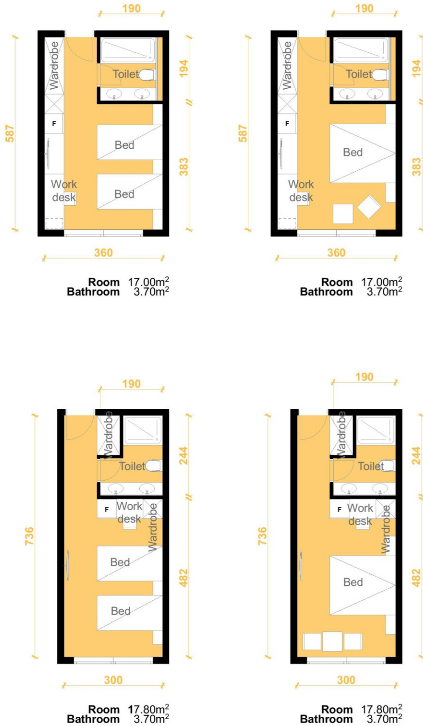
Figure 29 –Sample of the guestroom layout based on the minimum requirement set in Gazette (No.1963/28 of 20th April 2016) and Board Approved Guidelines.
