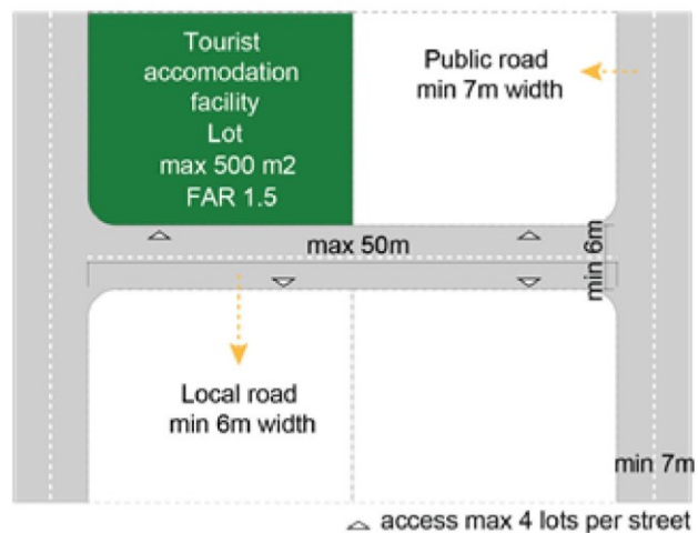
Figure 8 —Every such street shall connect on to a public street which is not less than 7m in width or a private street of which the owner of such private street has a right of way which is not less than 7m in width
