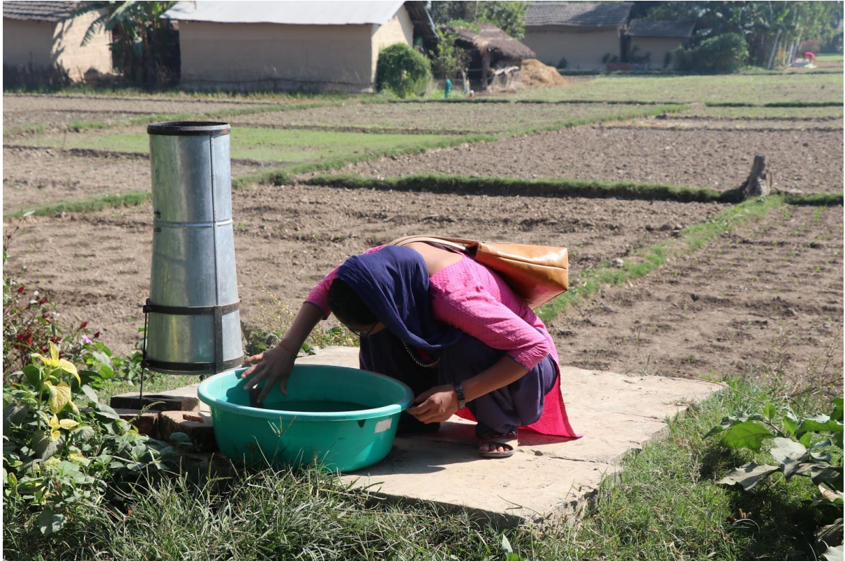
Figure 5-15: Local Field Assistant (LFA) recording evaporation and rainfall data in Kuti village.
