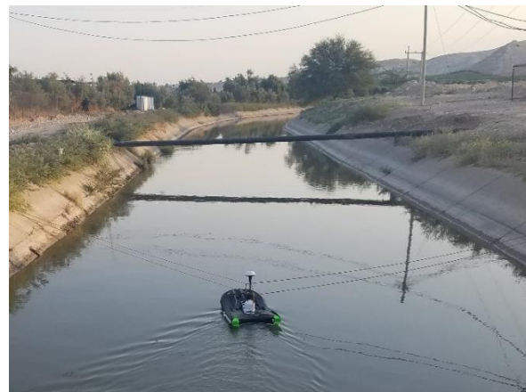
Figure 11: SonTek M9 instrument deployed on the KAC, July 2017
