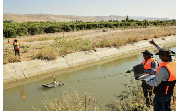
Figure 19: The SonTek M9 Operating on the KAC in July 2017
