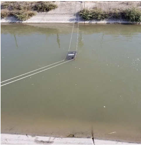
Figure 14: Deploying the SonTek IQ in the KAC, October 2017
