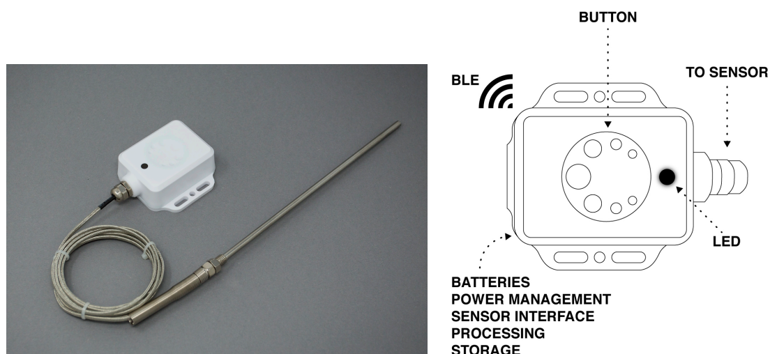
Figure 2. Geocene Dot. The left panel is a photograph of a temperature-logging Geocene Dot; the right panel is a schematic of the Dot. The Dot contains a BLE (Bluetooth Low Energy) radio for communication with mobile devices, a button to power on and power off the device, and an LED to indicate device status. The Dot requires two AAA batteries and includes power management, communication, and data processing and storage capabilities.
