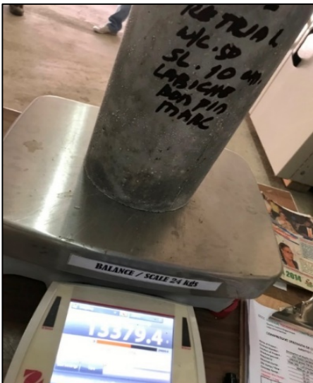
Figure 3.3.2-3. Concrete cylinder specimen no.2 weighted.
