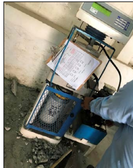
Figure 3.3.2-4. Concrete Cylinder specimen no.2 placed on the compression machine for the compressive strength test.
