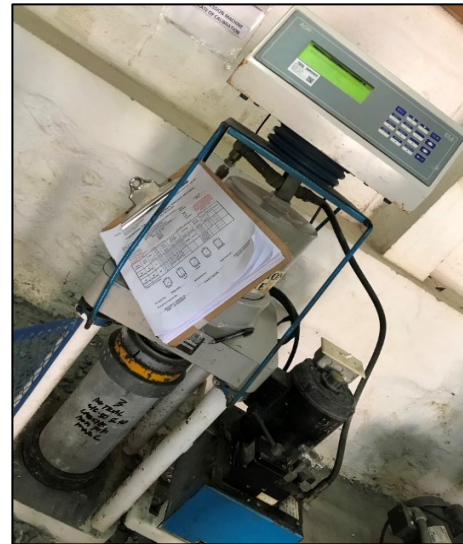
Figure 3.3.2-6. Concrete Cylinder specimen no.3 placed on the compression machine for the compressive strength test.
