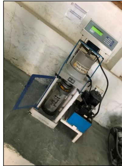
Figure 3.3.2-2. Concrete Cylinder specimen no.1 placed on the compression machine for the compressive strength test.
